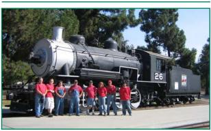
® Taking a short break from a big switching job, members of the museum's Train Operations Crew stopped to pose in front of Western Pacific locomotive No. 26. This ALCO 2-8-0 "consolidation" was built in 1909 and is Travel Town's largest steam locomotive - weighing in at 119 tons! From left: Greg Gneier, Vanya Holt, John Stumreiter, Greg Ramsey, Brad Slosar, Nancy Gneier, Craig Smith and Kevin Herrera.
