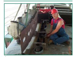
• Volunteer Kirk Reinholtz readies mounting brackets for the "exhaust deflector" unit, being installed on the roof of the Santa Fe M.177 motorcar.
